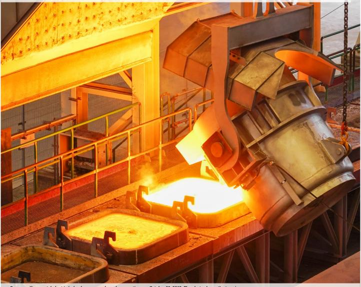
Our new silicon metal plant in Iceland commenced regular operations on October 30, 2019. The photo shows the teeming of the approximately 1,500 degree Celsius hot, liquid silicon metal into the casting frames, from which the metal is broken out after cooling and hardening. The metal is then further treated and prepared according to customer specifications.
