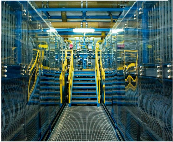
In 2015, we switched our entire chlorine manufacturing operation over to environmentally compatible membrane technology, with production being further expanded in the intervening years. At present, our annual capacity stands at 209,000 metric tons of chlorine and 236,000 metric tons of sodium hydroxide (chlorine co-product). We use most of the chlorine we manufacture as a feedstock for our own MCAA and propylene oxide production.
