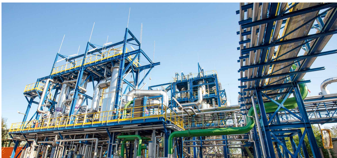
PCC Rokita SA again made a significant contribution to Group earnings in 2020. The photo here shows the modern membrane electrolysis plant used in chlorine production by this Group subsidiary in Brzeg Dolny.
